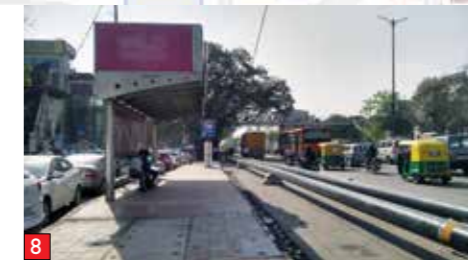
8 Bus stop covers the full width of the footpath
