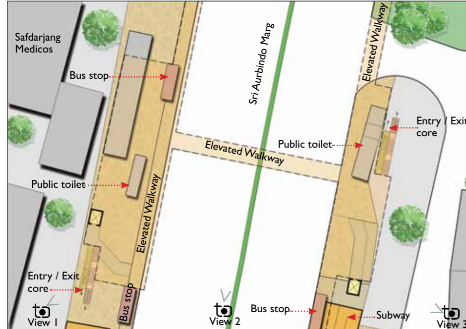
Grade level plan for the AIIMS Metro junction
