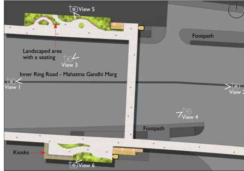
Elevated walkway level proposal for East Kidwai Nagar junction
